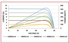
Average relative efficiency reduction of 5% at 200 W/m<sup>2</sup> according to EN 60904-1.
