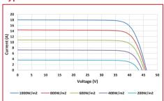
4) Average relative efficiency reduction of 5% at 200  $\mbox{W/m}^2$  according to EN 60904-1.
