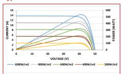
Average relative efficiency reduction of 5% at 200 W/m<sup>2</sup> according to EN 60904-1.
