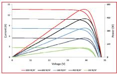
4) Average relative efficiency reduction of 5% at 200 W/m<sup>2</sup> according to EN 60904-1
