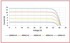
4) Average relative efficiency reduction of 5% at 200 W/m² according to EN 60904-1.
